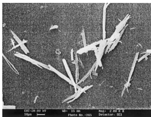
Figure 2 Wool fiber ground for 0.5 h (sample 2).
